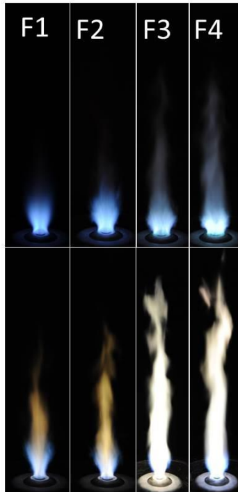
Figure 2: Direct flame images showing the effect of equivalence ratio at Re= 13,142 flames, top row without precursor and bottom row with precursor.
