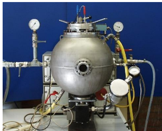
Figure 1: 20 litre sphere for the determination of the explosion indices LEL, P_{max} , K_{St}
