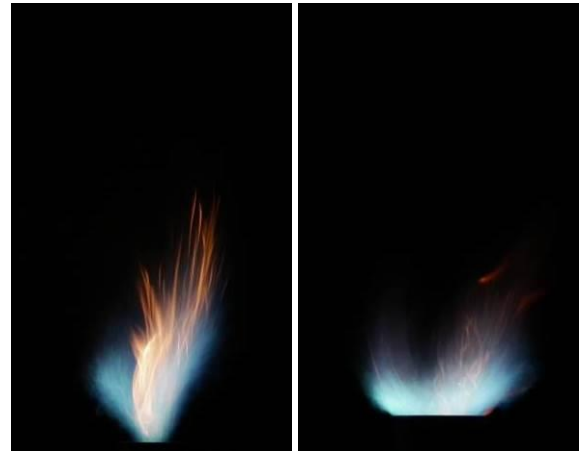
Fig. 5. Original (case B) and modified burner (case C) in operation at same operating conditions, 1/100 s, f/4
