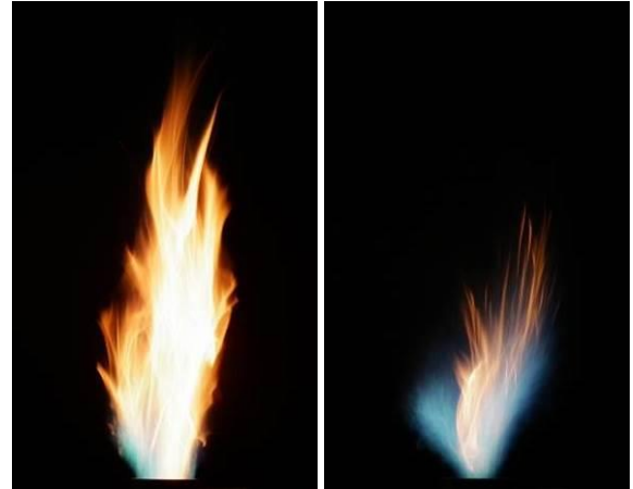
Fig. 3. Torch shaped (case A) and tulip shaped (case B) flame, 1/100 s, f/4
