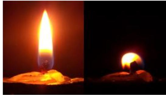
**Figure 6: Candle flame in normal gravity (left) and microgravity (right)**
