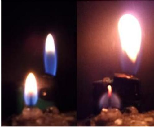
**Figure 9: Candle flame and ‘Cigarette Lighter’ flame in normal gravity (left) and microgravity (right)**
