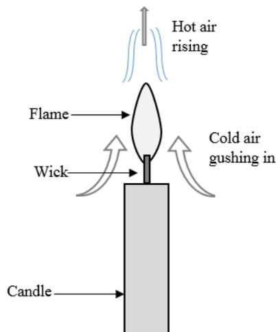
**Figure 5: Schematic of candle flame combustion process**
