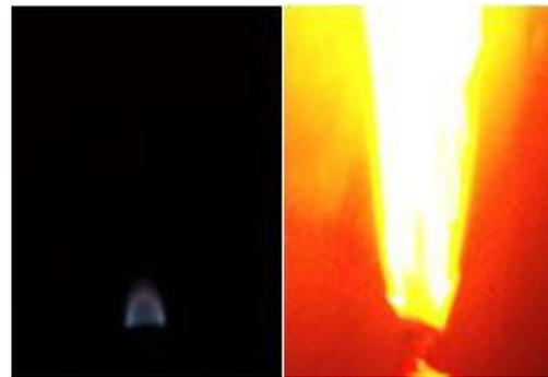
**Figure 8: Capillary based flame in normal gravity (left) and microgravity (right)**
