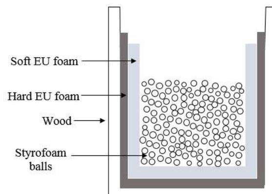
**Figure 4: Schematic of drop tower system**
