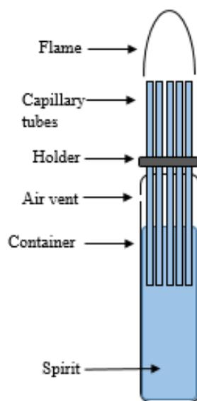
**Figure 7: Schematic of the experimental set-up of capillary based combustion**
