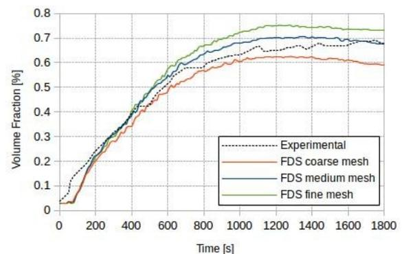
Fig. 7: Carbon dioxide volume fraction at position (9.0; 7.5; 3.5)
