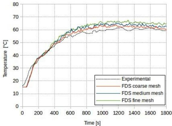
Fig 3: Experimental and numerical temperatures for the three grids at position (7.5; 5.0; 4.5)
