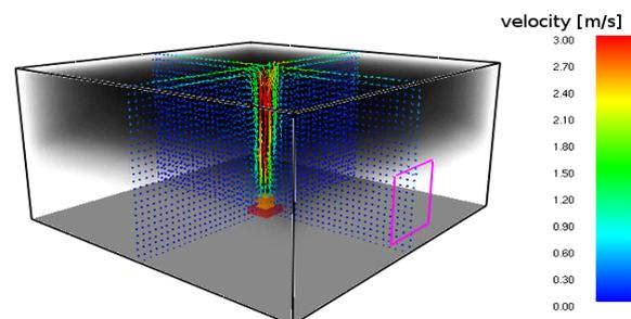
Fig. 1: Geometry of the test room, showing the smoke stratification and the velocity pattern
