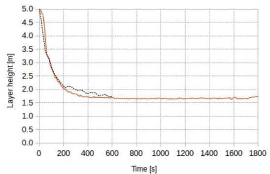
Fig 11: Smoke layer height comparison among experiment and simulation
