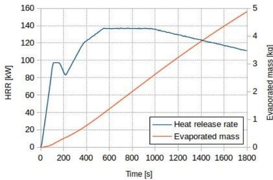
Fig. 2: Heat release rate and evaporated mass of heptane
