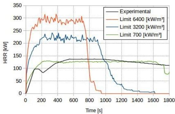
Fig 8: Heat release rate comparison for different limits of heat release rate per unit of volume
