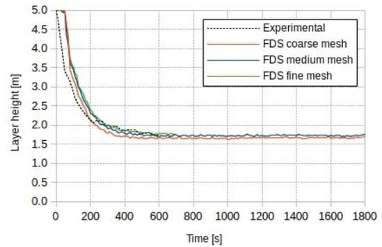
Fig 5: Smoke layer height calculated using Eq. 5 for the different grids
