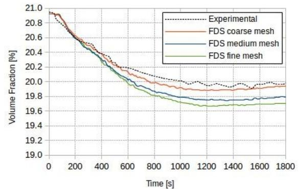
Fig. 6: Oxygen volume fraction at position (9.0; 7.5; 3.5)
