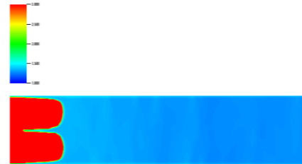
Figure 3 Temperature distribution ahead of the flame
