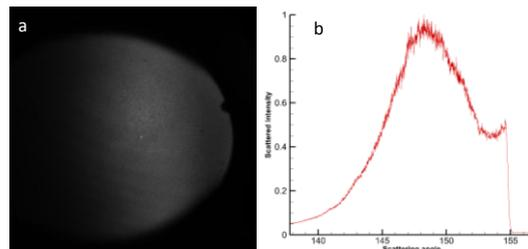
Figure 3 : Experimental global rainbow technique. Image of the rainbow signal (a). (b) Evolution of the intensity as a function of the scattering angle.
