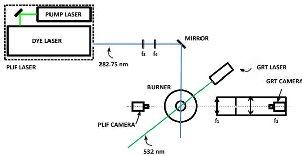
Figure 2 : Schematic representation of the dual measurement technique.
