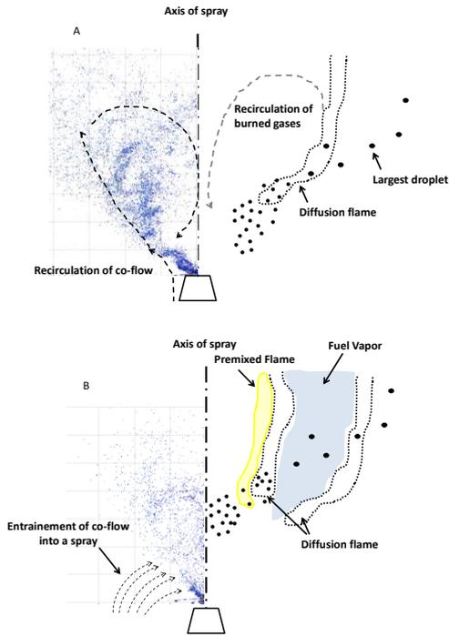
Figure 9: Schematic double flame structure with swirl (A) and without swirl (B)
