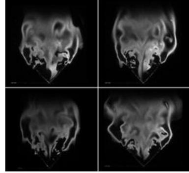
**Figure 7:** Single-shot OH-PLIF images for hollow cone pressure-swirl nozzle with 3.00 g/s co-flow with swirl.
