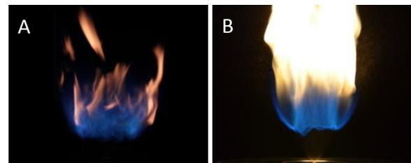
Figure 5 : Image of spray jet flame without swirl (B) and with swirl (A)
