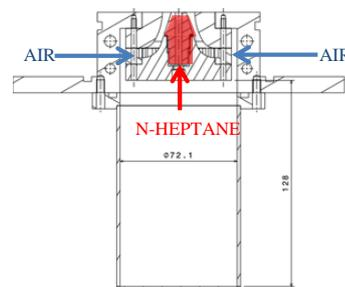
Figure 1 : Combustion Chamber. Blue: laminar coflow (air). Red: fuel injector.
