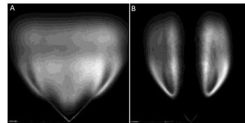
**Figure 8:** Average images of OH PLIF for two configurations : (A): With swirl and (B) : without swirl
