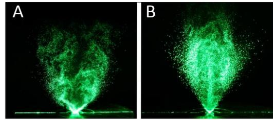
Figure 4 : Fuel droplet Mie scattering A: Configuration with an Air/swirl in the system of co-flow of air B: Configuration without swirl
