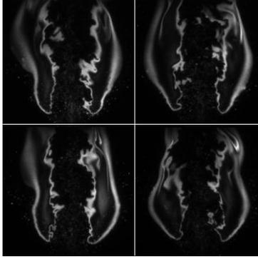
**Figure 6:** Single-shot OH-PLIF images for hollow cone pressure-swirl nozzle with 6.00 g/s co-flow.
