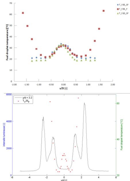
Figure 11: Evolution of fuel droplet temperature
