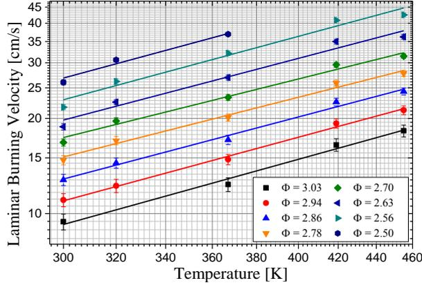
**Figure 6: Double logarithmic diagram of laminar burning velocities of investigated equivalence ratios at different preheating temperatures**
