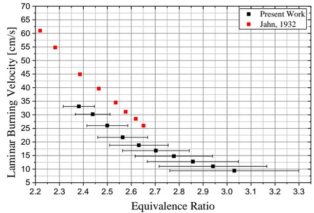
**Figure 4: Laminar burning velocities of fuel-rich methane oxygen Mixtures at  $T_p = 300$  K and ambient pressure**
