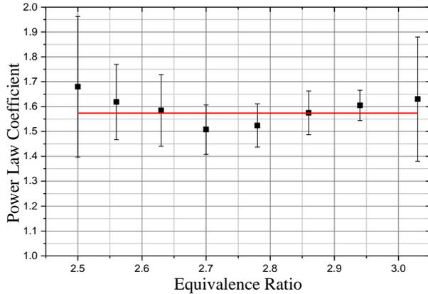
**Figure 7: Determined power law coefficients  $\alpha$  at investigated equivalence ratios**
