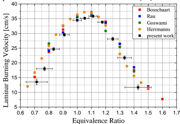
**Figure 3: Laminar burning velocities of methane air mixtures at  $T_p = 300$  K and ambient pressure**
