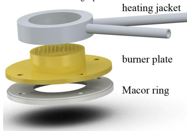
**Figure 2: Parts of the burner head**
