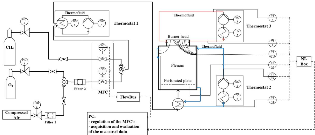
**Figure 1: Piping and Instrumentation Diagram of the Test rig**
