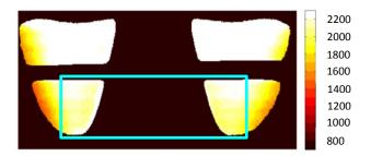
Figure 5: Example of a temperature field (in Kelvin) obtained with the 2-color OH-PLIF technique for a premixed stoichiometric CH<sub>4</sub>/air flame.
