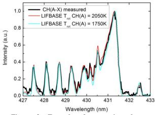
Figure 3: Example of comparison between measured CH (A-X) spectra and simulations performed with LIFBASE [10].
