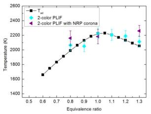
Figure 8: Comparison of temperatures of flames and temperatures of flames enhanced by NRP corona discharges, measured by 2-color OH-PLIF.
