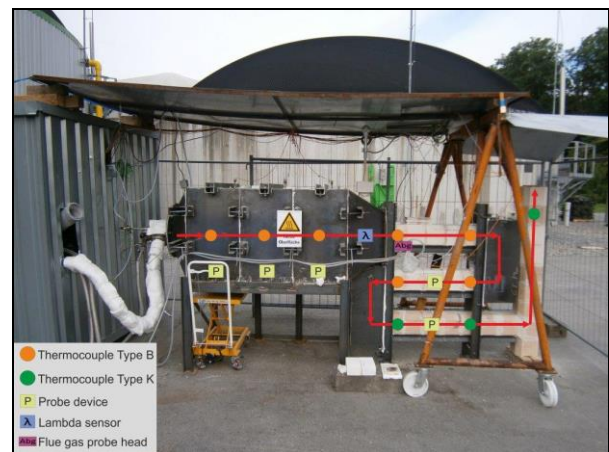
Figure 6: Mobile test rig with measurement positions
