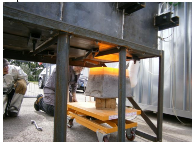
Figure 7: A crucible containing a glass batch sample is inserted into the furnace
