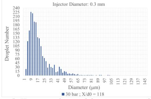
Figure 5: Histogram for one 0.3 mm injector at 30 bar water pressure
