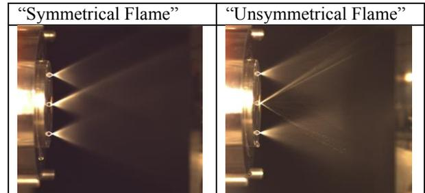
Figure 15: Potential relation between the jet quality of impingement and the flame structure
