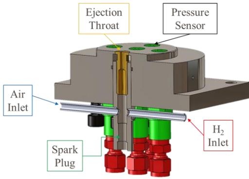
Figure 7: The torch igniter inserted in an available slot of the injector plate
