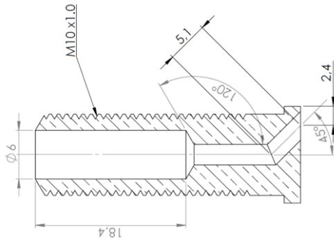
Figure 9: The inclined ejection throat
