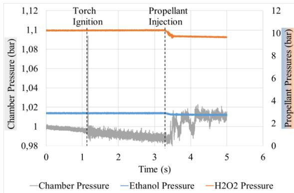
Figure 12: Pressure signals in the chamber and for the propellants (test n°1)
