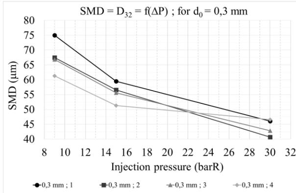
Figure 6: SMD as a function of water injection pressure for 4 injectors of 0.3 mm diameter
