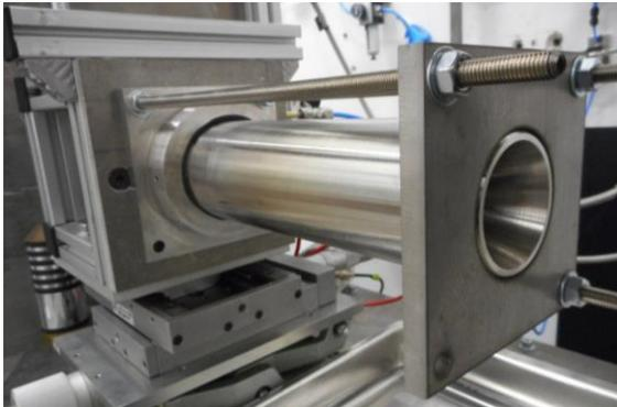
Figure 2: The combustion chamber before the experiments
