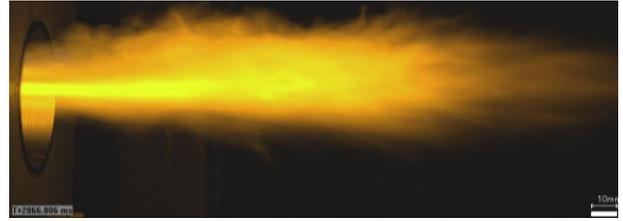
Figure 14: Unsymmetrical flame (conditions of test n°2)
