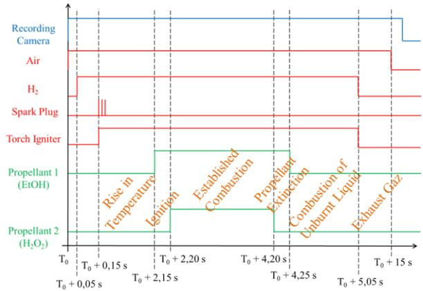
Figure 10: The short-time propellant injection chronogram
