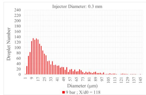
Figure 3: Histogram for one 0.3 mm injector at 9 bar water pressure
