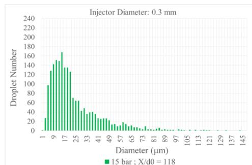
Figure 4: Histogram for one 0.3 mm injector at 15 bar water pressure
