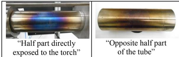
Figure 18: Combustion chamber after the series of experiments (temperature distribution)
