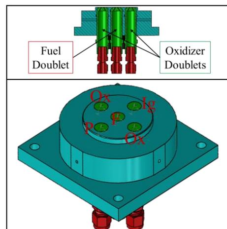
Figure 1: The injector plate fitted with injectors of oxidizer (Ox) and fuel (F), and the slots for the torch igniter (Ig) and the pressure sensor (P)
