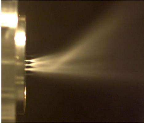
Figure 8: The effect of the torch igniter on the central spray (non-reactive conditions)
