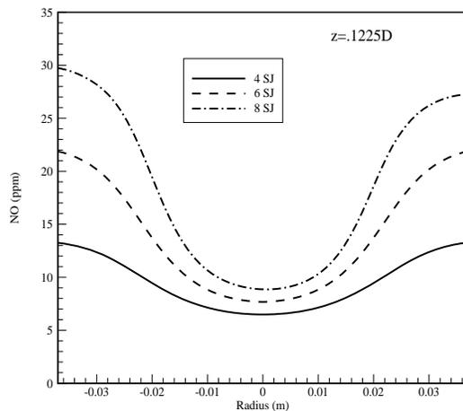
Figure 7. Effect of stabilizer jet holes number on NO concentration distribution at various axial distance
