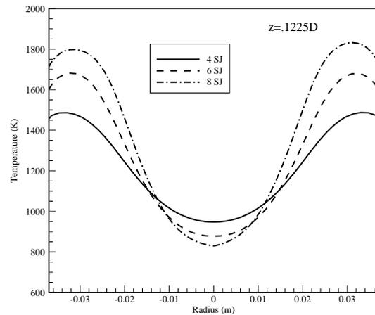
Figure 5. Influence of stabilizer jets number on temperature distribution at  $z=1.225D$
