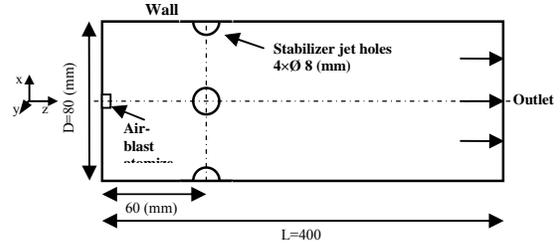
Figure 1. Schematic view of model combustion chamber
