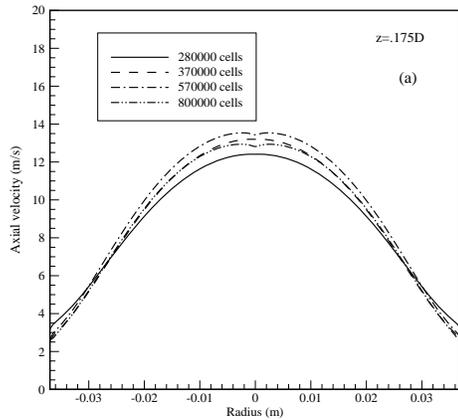
Figure 2. Independence of present computations from mesh size: axial velocity and at  $z=1.75D$
