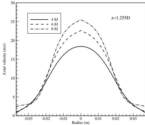
Figure 6. Influence of stabilizer jets number on velocity distribution at  $z=1.225D$
