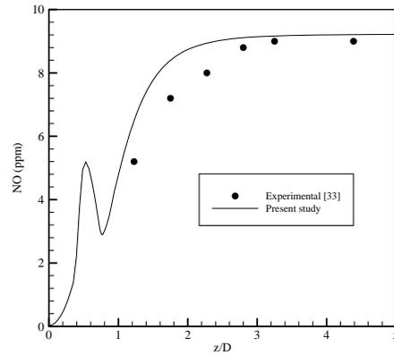
Figure 4. Variation of NO concentration with axial distance (center-line,  $x=y=0$ )
