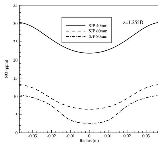
Figure 9. Effect of stabilizer jets position (SJP) on NO concentration distribution at  $z=1.225D$
