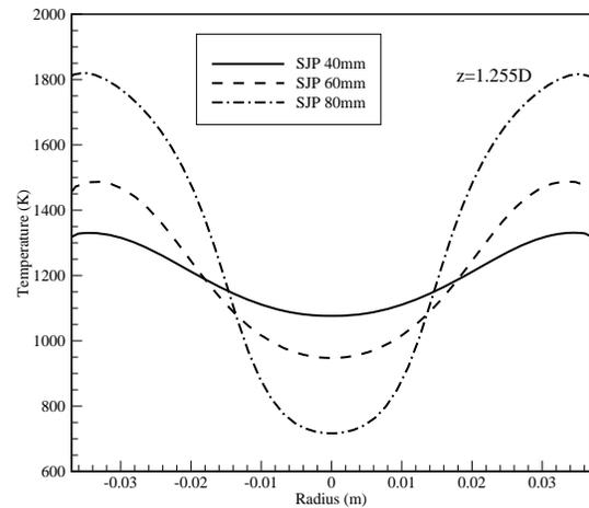
Figure 8. Influence of stabilizer jets position (SJP) on temperature distribution at  $z=1.225D$
