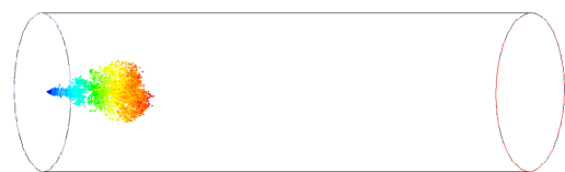
Fig.4. Predicted spray pattern of numerical spray model (t=0.2ms).
