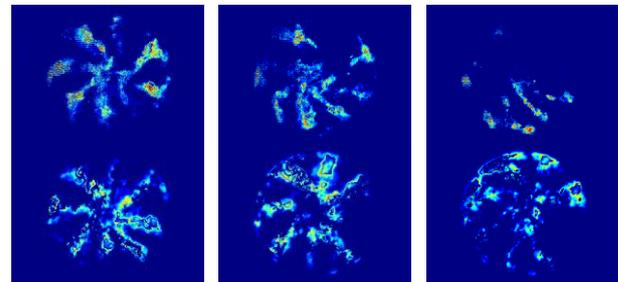
**Figure 10 Comparison between CH (upper) and  $C_2$  (lower) chemiluminescence signal for Case B for 7.6, 10.1 and 13 CAD subsequently**
