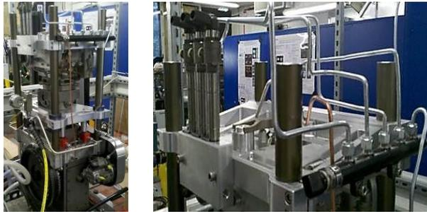
**Figure 4 Ricardo Hydra single cylinder optical engine sharing the same cylinder head geometry as the metal Ford engine**
