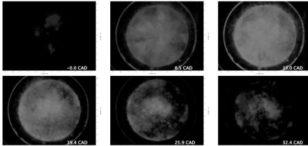
**Figure 7 High speed flame luminosity measurements for Case B, i.e. triple injection strategy employed.**
