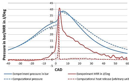
**Figure 11 Pressure and heat release experimental data comparison with numerical predictions of a three zone combustion model.**
