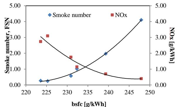
Figure 3  $\text{NO}_x$  and smoke levels (%) measured
