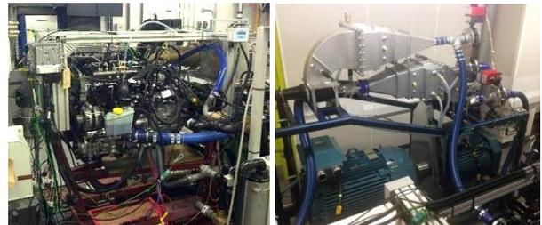
Figure 2 Ford Puma engine and electrical boost unit
