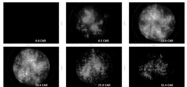
**Figure 5 High speed flame luminosity measurements for Case A, *i.e.* triple injection strategy employed.**
