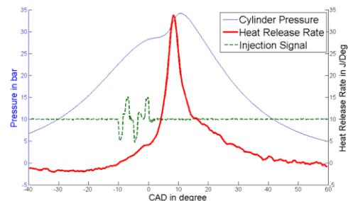
**Figure 6 In-cylinder pressure, calculated heat release rate and injector signal for Case A.**
