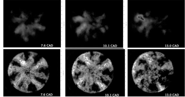
**Figure 9 Comparison between Cases A (top) and B (bottom) via  $C_2$  chemiluminescence imaging**
