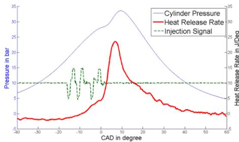
**Figure 8 In-cylinder pressure, calculated heat release rate and injector signal for Case B.**
