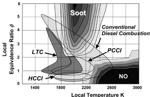
Figure 1 LTC and PCCI concept on  $\phi - T$  map [18]
