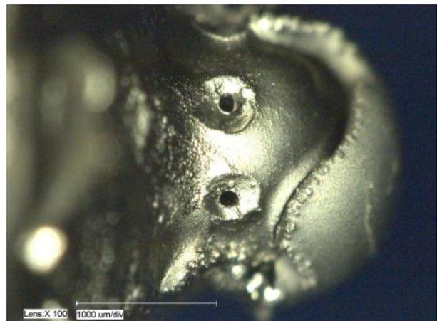
Figure 3: External deposits after test run (1,300 bar, 10 Hz, 500  $\mu$ s, B10)
