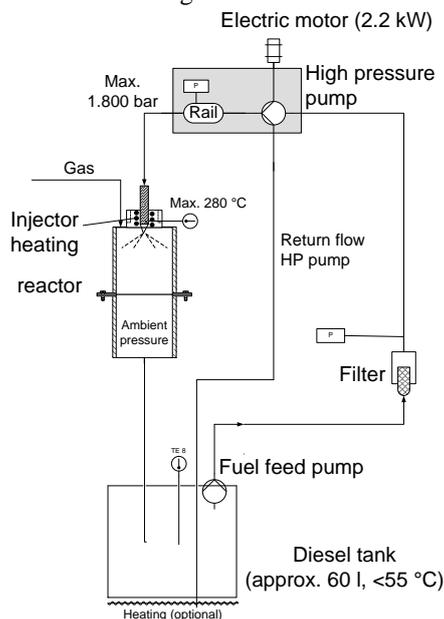
Figure 1: Flow sheet of one common rail system on the test rig.
