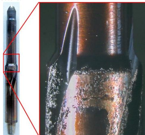
Figure 2: Deposits on the injector needle
