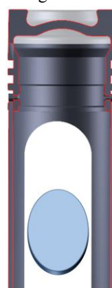
Figure 1 Elongated piston and 45° mirror
