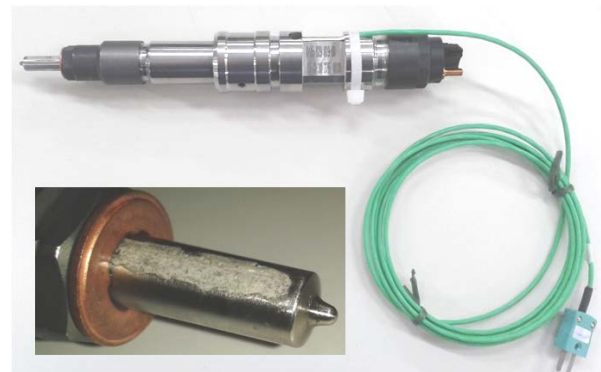
Figure 4 - Common rail injector instrumented for NTT measurement
